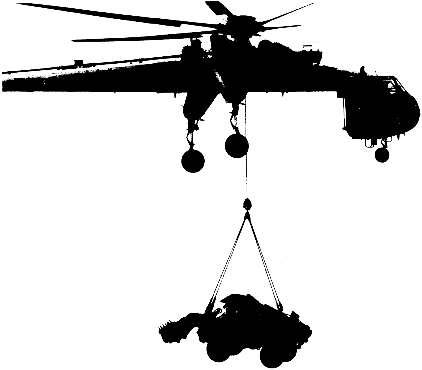
Figure 4-6. SEE being lifted by CH-54 helicopter.
